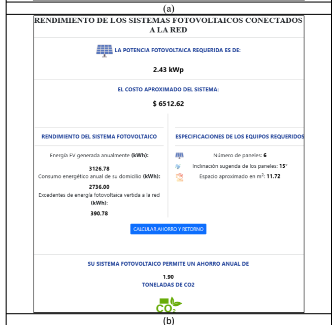
Fig. 6. Design of the secondary side for the calculation of the sizing of photovoltaic systems based on their consumption. (a) Input screen, (b) Simulation result
