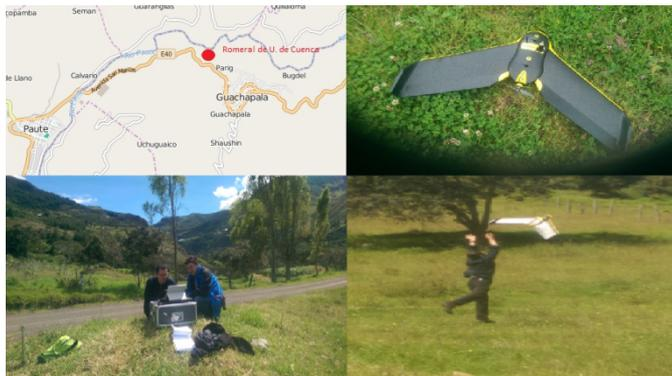
Fig. 2. Location of the Romeral of the University of Cuenca. VANT eBee RTK. Configuration of the flight through the software emotion. Drone's launching.
