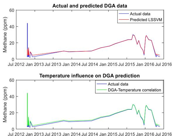
Figure 8 Methane time-series comparison between DGA forecasting model and temperature correlation model
