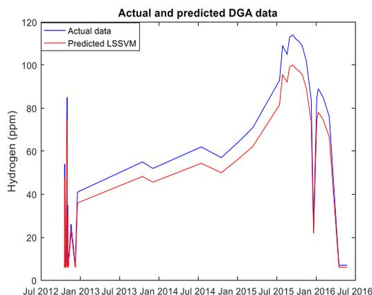
Figure 5 Actual and predicted DGA data using LSSVM model – hydrogen
